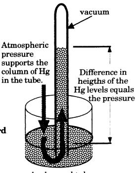
beaker and tube filled with Hg
