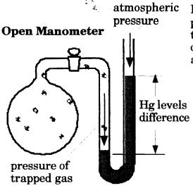
In the open manometer at the left, the trapped gas pushes down on one side of the mercury in the bent tubing while the atmosphere pushes down on the other side of the tube. The gas pressure equals the atmospheric pressure ± difference in Hg levels.
