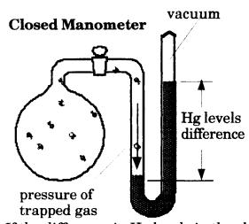
In the closed manometer at the left, the trapped gas pushes down on one side of the mercury in the bent tubing while there is **no gas** pushing down on the other side of the tube. The sealed end of the tubing contains a vacuum, which exerts no pressure by itself. Only the weight of the Hg column creates any pressure on the side of the sealed tube. Therefore, the pressure of the trapped gas equals the height of the Hg column that it can support(the difference in the Hg levels).
